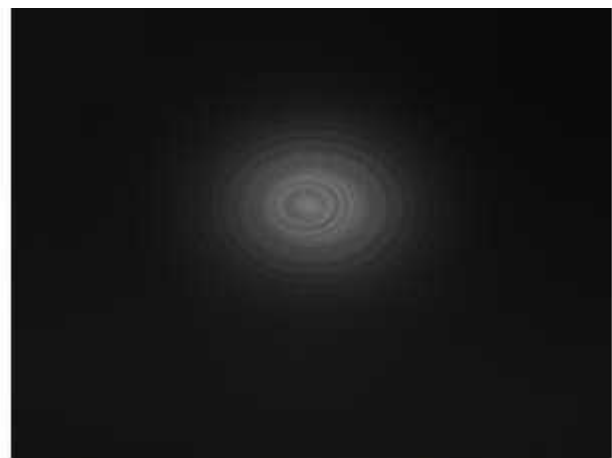
Light emerging from a single mode fiber
